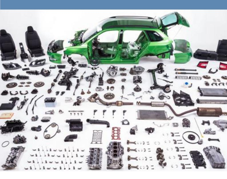
Disassembly of a ŠKODA FABIA COMBI 1.2 TSI DSG after it had covered over 100,000 kilometers in a long-term test by the German magazine Auto Bild.
